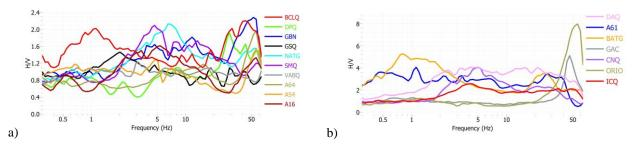
Figure 3. Time-averaged MHVSR amplification spectra from single-sensor measurements performed beside the CNSN seismograph for sites with (a) relatively 'flat' (< 2) amplification and.(b) a clear broad or sharp MHVSR peak.
