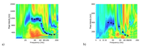
Figure 5. MASW dispersion histogram for (a) station QCQ with observed phase velocities (> 1000 m/s) of underlying rock and (b) station DAQ with observed phase velocities (< 400 m/s) of shallow sediments.
