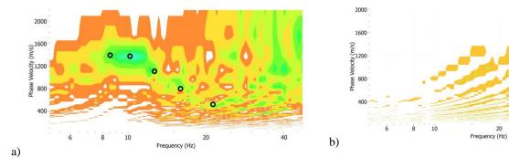
Figure 4. Two cases of MSPAC dispersion histograms from AVA recordings at station (a) station OTT with retrieved dispersion estimates (open circles) and (b) station NATG showing no success in measuring dispersion.
