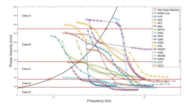
Figure 6. Dispersion estimates from active- and passive-source array methods. Solid black line shows Vr40 with converted Vs30-to-Vr40 site class boundaries denoted as stars and labelled.
